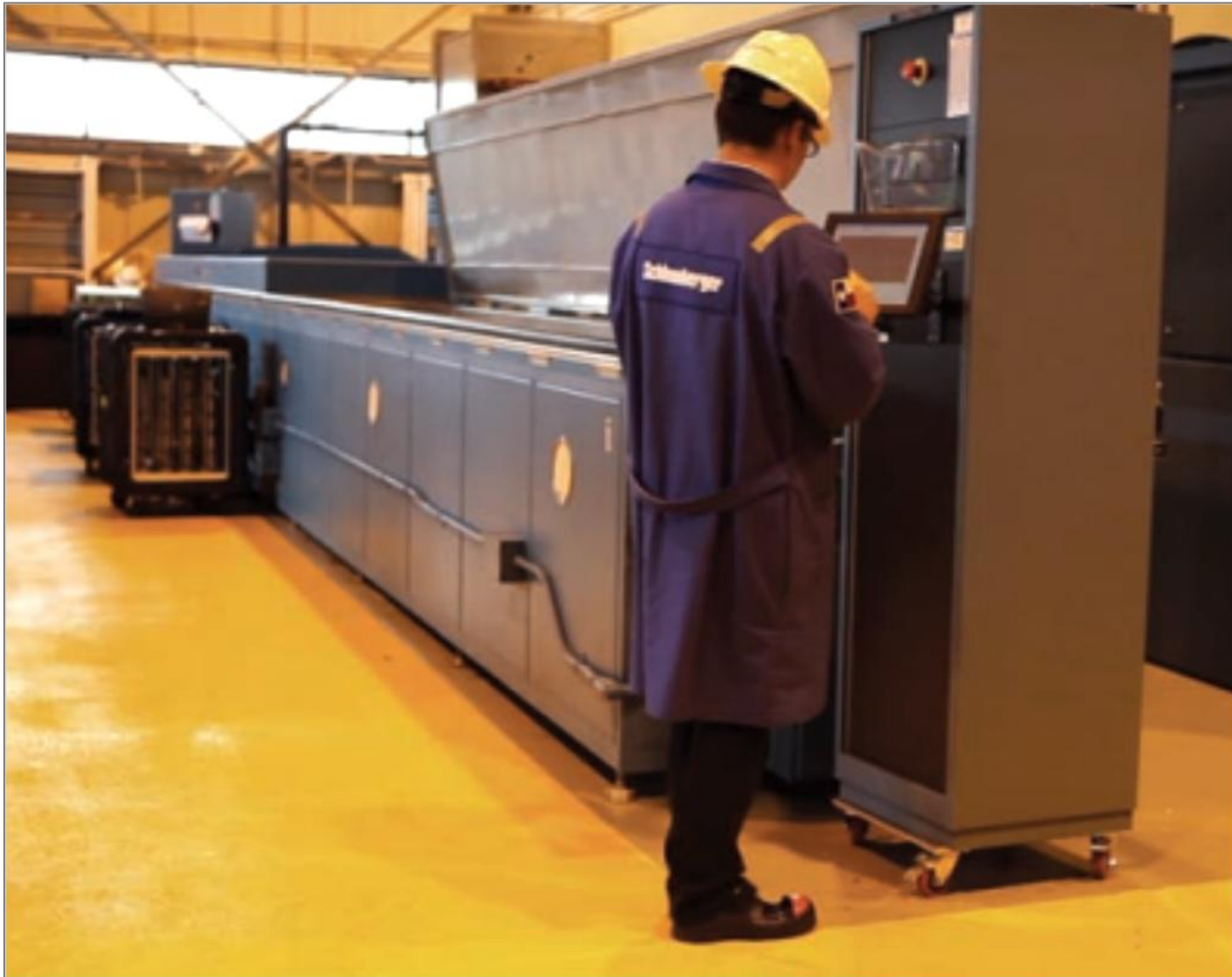
Figure 6. MDT-Forte-HT modules are tested as temperature extremes including thermal cycling and aging and high-temperature life.
